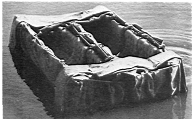
Figure 4. Two halves of the boat are lashed together down the center footrests.
