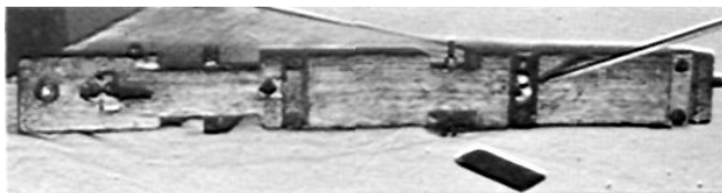
Figure 3—To bore-sight the piece, the mount is designed to permit elevation and depression of the muzzle. This is done by drilling a vertical hole in the block, inserting a 5\frac{1}{2} " \times \frac{3}{4} " machine bolt, welding a 1\frac{1}{4} " threaded portion of another machine bolt to the 37-mm bracket, and adjusting the angle of elevation of the mount by use of a 1\frac{1}{4} " \times \frac{3}{8} " hexagonal connecting nut.
